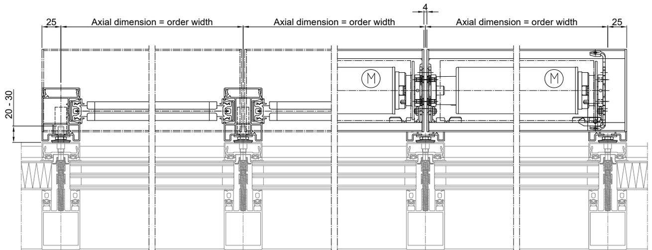
The greyed-out sections of the illustration represent interfaces to general trades which, on the whole, must be planned and performed independently and on-site. WAREMA does not provide services for the greyed-out interfaces and assumes no liability for them.
