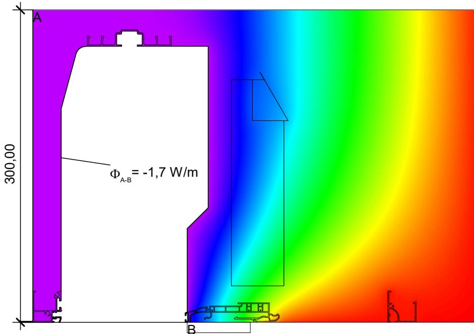
$$U_{SB\ A-B} = \frac{\Phi}{\Delta T \cdot b} = \frac{1,651}{20,000 \cdot 0,300} = 0,275 \text{ W}/(\text{m}^2 \cdot \text{K})$$
