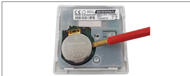
Fig. 5 Removing the battery
