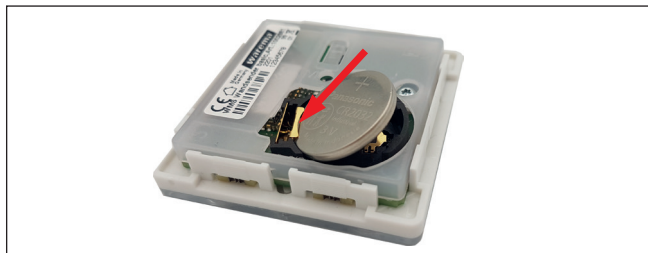
Fig. 6 Inserting the new battery
