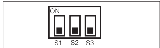
Fig. 1 factory setting encoding switch
